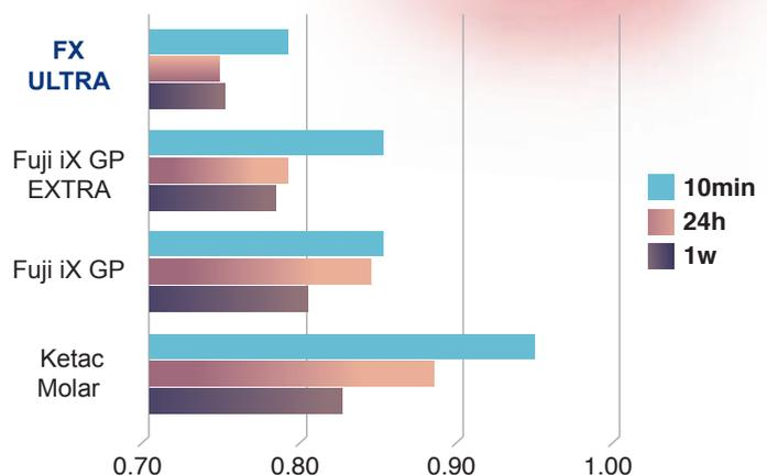
Contrast Ratio (10min, 24h, 1w after start of mixing)
